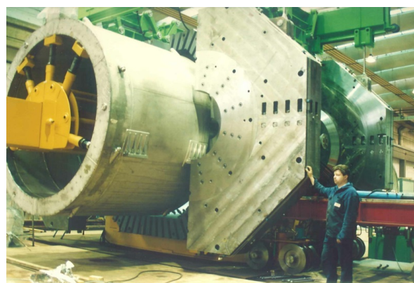
Test of insertion of complete magnet inside magnetic yoke
